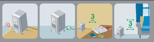
Check your space heater for cracked or damaged cords and plugs. Plug space heaters directly into wall outlets, don't use an extension cord or power strip.
